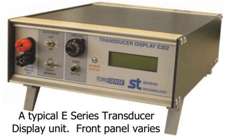
A typical E Series Transducer Display unit. Front panel varies depending on model.
