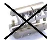
2. **For Transducers below 1Nm or 10lbf.in** or if the application requires the body to be **rigidly mounted** then it is recommended that double couplings should be used at each end to compensate for any misalignment of the input/output shafts and the system designed to eliminate any end loads on the transducer shaft. For applications where **end loads cannot be avoided** please consult the ST sales department for advice **prior to ordering**.
