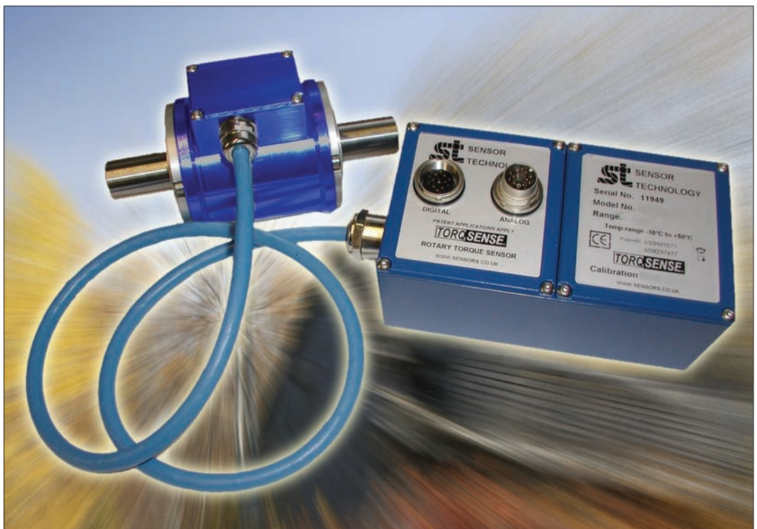
Fig. 1. The digital TorqSense unit emits a low powered radio frequency signal towards the piezoelectric acoustic wave combs which are reflected back to the unit.
