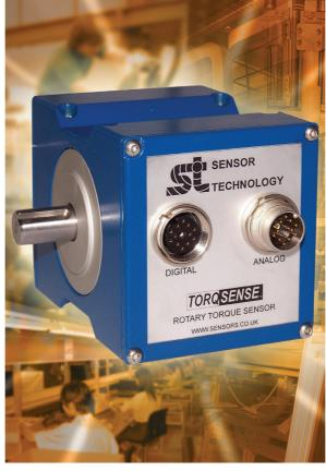
The devices are fixed onto a shaft to form part of a high frequency oscillator circuit: each device is angled at +45° to the axis of the shaft. When the shaft rotates under load it deforms by twisting: this compresses one SAW device and stretches the other, each allowing their resonant frequency to alter and thus changing the frequency difference between them. This difference in the two frequencies is a measure of the induced strain due to the twisting moment and
