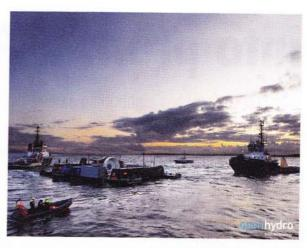
OpenHydro deployed its first commercial-scale in-stream tidal turbine in the Bay of Fundy, Canada, on behalf of its customer, Nova Scotia Power. This 1MW unit was operational, rotating with the tides, collecting data and producing energy just a week after arriving on site
