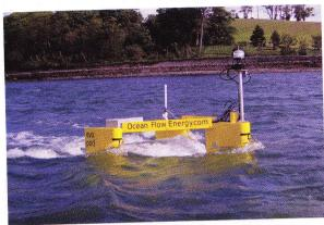
Evopod is a semi-submerged, floating, tidal energy capture device
