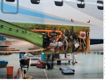
Every modern aircraft has at least one on-board generator to produce electrical power, although most have two or more in a redundancy configuration for utmost reliability. These need to be ground tested regularly, typically every 500 to 1000 flying hours.
