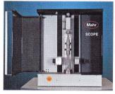
Capable of measuring turned parts up to one metre long by 120mm diameter and weighing up to 30kg, the MarScope available from **Mahr UK** is designed to operate both in the laboratory and on the shopfloor. It
