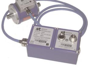
cipal requirement is to measure the torque in a shaft while it is rotating, often at high speed.
