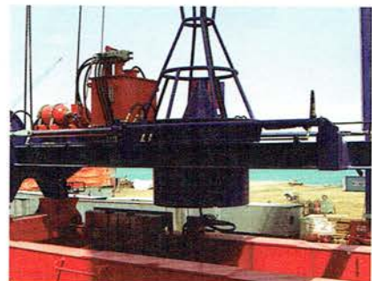
The Ruppel system allows the amplitude, and therefore the oscillation period of a container, to be reduced.
