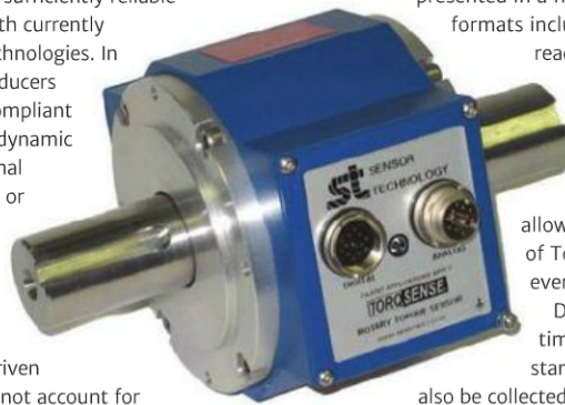
The principle behind SAW devices used in TorqSense transducers is that they are essentially 'frequency dependent' strain gauges, which measure a change in SAW resonant frequency caused by an applied shaft strain
