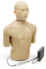
time. Produced from soft silicone, the concha and canal of the pinna have been modified so that they closely mimic the properties of a human ear. *Stand C3*
