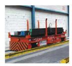
for transferring materials between buildings where craneage is not available or for moving stocks long distances to despatch rather than tying up a forklift for this bulk task
