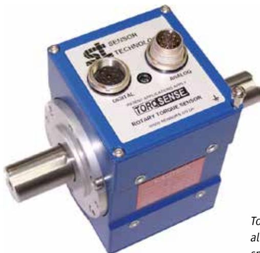
*TorqSense from Sensor Technology meets all criteria: simplicity, robustness, high speed and wireless*
