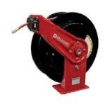
Reelcraft's new Series HD70000 hose reels are designed to accommodate up to 30 m of 6 mmm I.D. hose or 23 m of 13 mm I.D. hose. The heavy duty base design, all steel construction and a baked-on powder coat finish combine to produce a rugged, corrosion-resistant product. A
