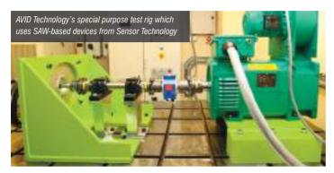
Wireless rotary torque transducers from sensor supplier, **Sensor Technology** are at the heart of a test rig to develop next generation technologies for electric and hybrid vehicle powertrains. With unique expertise in the electric motors and electronics used across the key powertrain technologies, AVID Technology relies on the innovative torque transducers as part of an automated approach to motor characterisation
