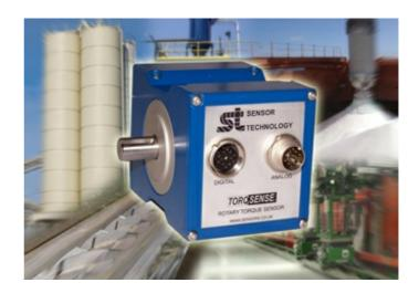
Electronics convert the data stream directly into engineering outputs, such as torque, speed, power and angle. Serial and USB interfaces make TorqSense directly compatible with PCs and other user-friendly features include built-in peak torque sampling, storage and torque averaging, and a self-diagnostics test package. The electronics can be provided, integral with the main unit or in a separate housing, to suit individual applications.
