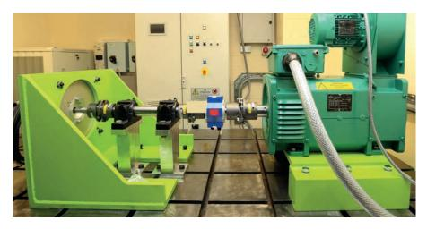
Avid Technology is relying on innovative torque transducers in its automated test rig for electric motors
