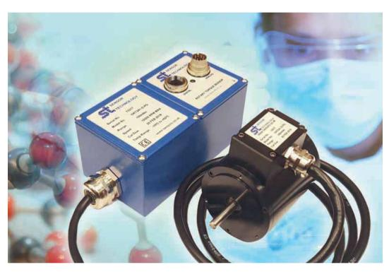
TorqSense is unlike any other sensor in that it does not rely on delicate slip rings to transmit torque readings. It does this wirelessly using radio signals transmitted from a pick-up located near to, but not actually contacting the rotating drive shaft of the capping mechanism. TorqSense met the design criteria of robustness, simple high-speed operation and non-contact for sterility.
