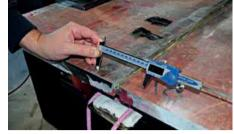
is required to identify any discontinuities in the welding profile, including careful measurement of weld shrinkage. This careful evaluation of the weld will determine acceptance or rejection depending on the required criteria.
