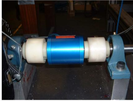
**Figure 1.13.** Photograph of torque transducer installed on shaft.
