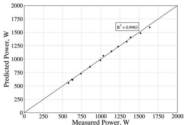
**Figure 8. Compares the full flow measured power for the dual rotor fitted with the standard hole emulsifier screen with the line predicted from a multilinear regression fit to a large matrix of experiments on the same set-up.**
