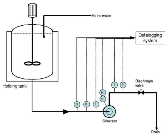
**Figure 1. Schematic of experimental rig.**
