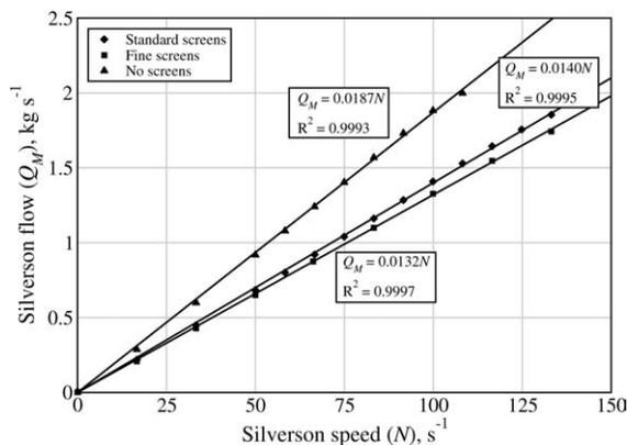
**Figure 5. Silverson 150/250 MS with the dual rotor showing unfettered flow for three different stator screen arrangements—The standard dual emulsifier mesh; the fine emulsifier mesh and with no screens.**
