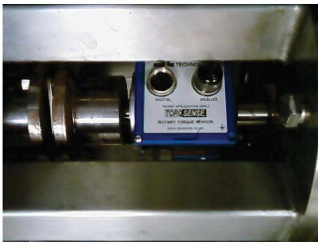
**Figure 4. TORQSENSE torque meter fitted to Silverson drive shaft.**
